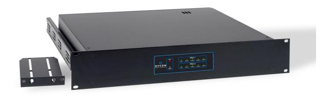
The Dycon D1438-DR 2U PSU is a high end, fully-monitored, switched-mode power supply with processor controlled reset. The unit is suitable for use in a 19" computer rack and is supplied as standard with brackets and full-extension sliders. The 2U-size unit includes an integrated hinged tray providing space for third-party control units e.g. Lenel™ or Mercury™ or Vanderbilt™ system/door controllers.
